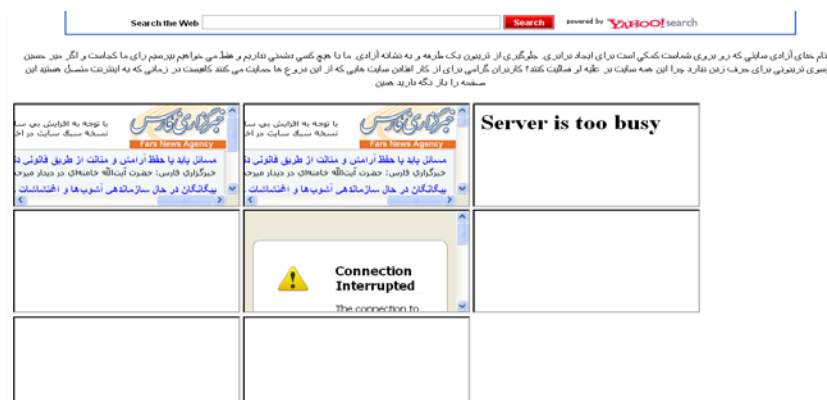
Figure 5: Example of a denial of service attack page serving multiple framed instances of the targeted website, and responses from the server indicating their relative success.
