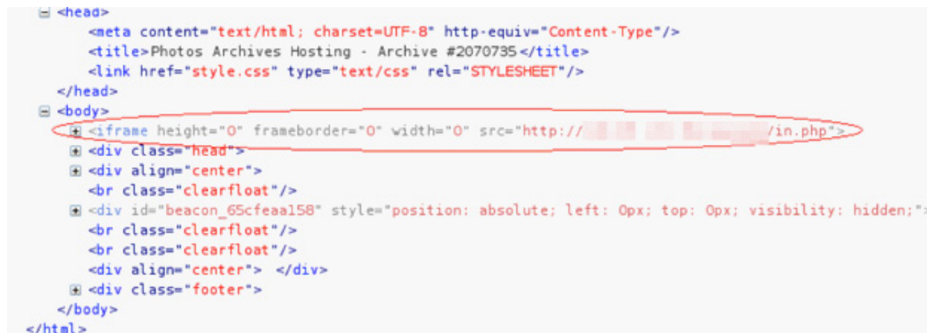
Figure 23: Hidden iFrame Pulling in Content from a Remote Server Hosting an Exploit Kit
